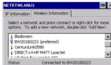
Figure 3 — Select the BWxxxxxxxx entry and click the Advanced button to set the parameters.
