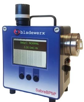
reliable 1024-channel multichannel analyzer provides input for an embedded processor board to perform beta detection and alpha spectral analysis for radon background compensation. An internal gamma guard detector provides real time beta channel compensation for changing ambient gamma background levels. An integrated 7-LPM pump, lithium-ion battery and charging electronics complete the package allowing for battery operation of up to eight hours.
